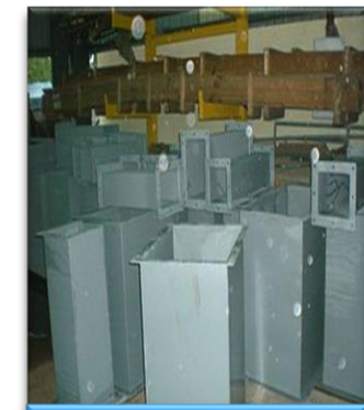
Mild Steel Penetration Ducting
